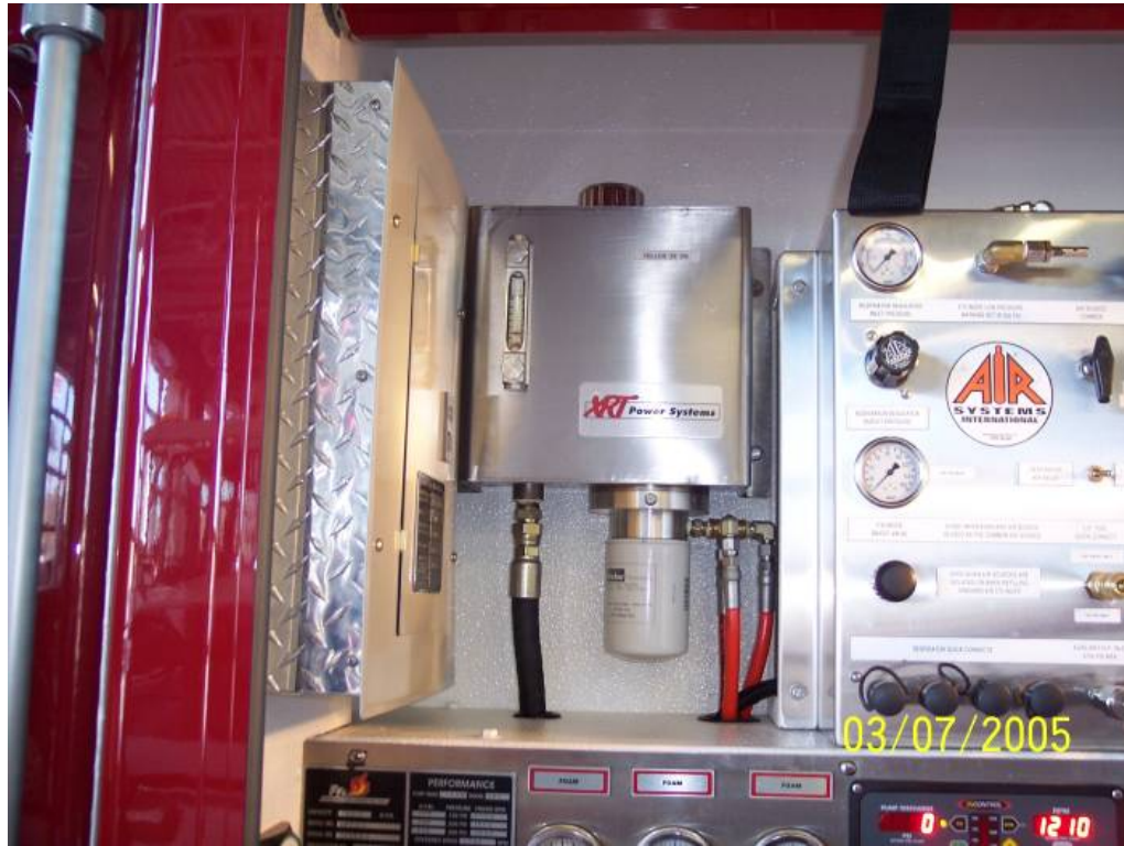
Photo 1 - Oil Reservoir Tank
